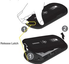
Place your fingernail into the Release Latch indention (adjacent to the microphone) and carefully lift (1) the case off the rear of the phone (2).
